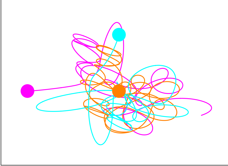
Fig. 1: Example of the trajectories for 3 equal mass bodies interacting gravitationally, generated by solving the equations of motion numerically. The filled circles indicate the initial positions of each mass, distinguished by each having a different color in the picture. A very slight modification of the initial conditions can lead to very different trajectories, a generic feature of chaotic systems.
