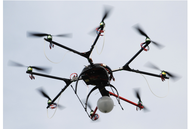
Figure 3: Octocopter with light source. The eight engines of the octocopter are arranged on a circle. Their supporting rods are connected to a central platform carrying all circuit boards for operation and communication. The light source is attached to the supporting rods of the two engines that define the forward direction.
