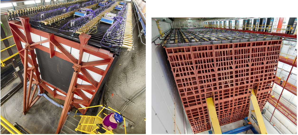
Figure 3.7: The NOvA Detectors. The NOvA near (far) detector on the left (right).
