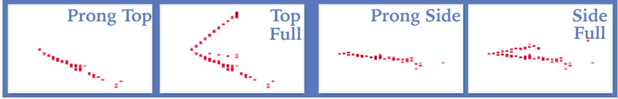
Figure 5.8: Prong Classification Inputs. The 4 arrays used as input to the network for particle classification. The left two inputs are the X-view of the prong and full event respectively. The right two inputs are the Y-view of the prong and full event respectively.
