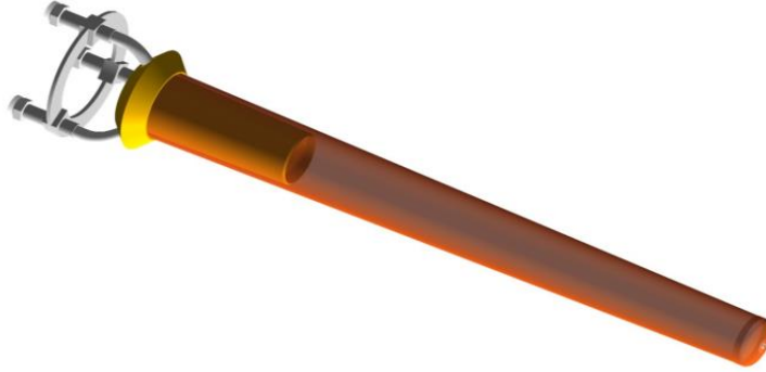
Figure 3.8: Kapton container for the liquid deuterium target [21]
