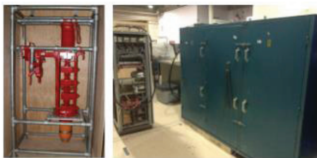
Figure 4: 1.3 GHz klystron and modulator system at CSU.
