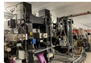
Figure 10: Photo of CPMU-4 installed in I04 beamline.
