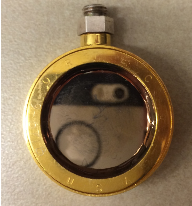
FIGURE 3.11: (Color online) The front surface of the SSB T-type detector. The reflective surface is the silicon wafer coated with a very thin layer of gold. The wafer is encased into a cylindrical Faraday cage and connected to a microdot connector.
