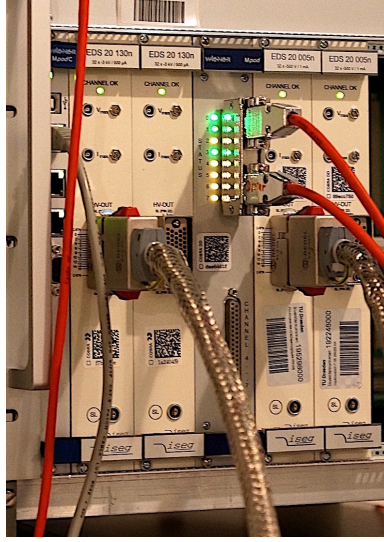
Figure A.18: MPod crate with installed high voltage modules (EDS 20 130n, slot 1 & 2), grid bias modules (EDS 20 005n, slot 4 & 5) and low voltage modules (Wiener-LV-Modul 8008). Low voltage module supplies the preamplifier boxes and the dewar heater.
