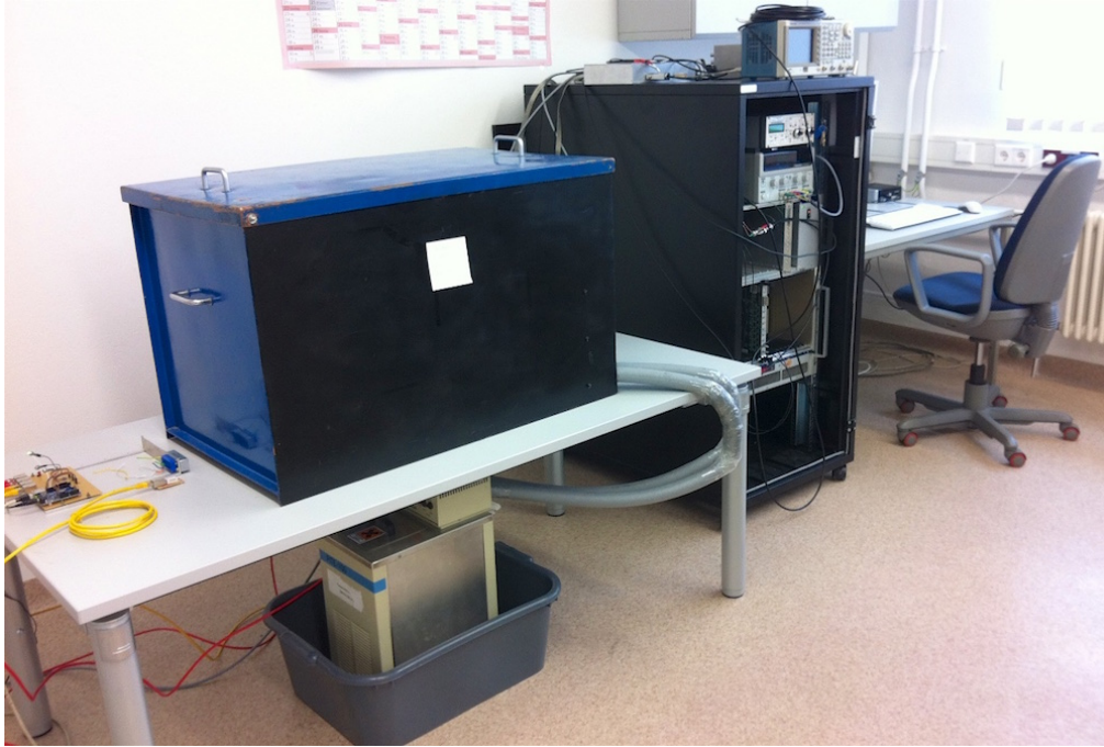
Figure 3.12: The thermal isolated cooling box on the table, chiller device below the table, electronics rack with power supply, pulser, FADCs, computer on right hand side.
