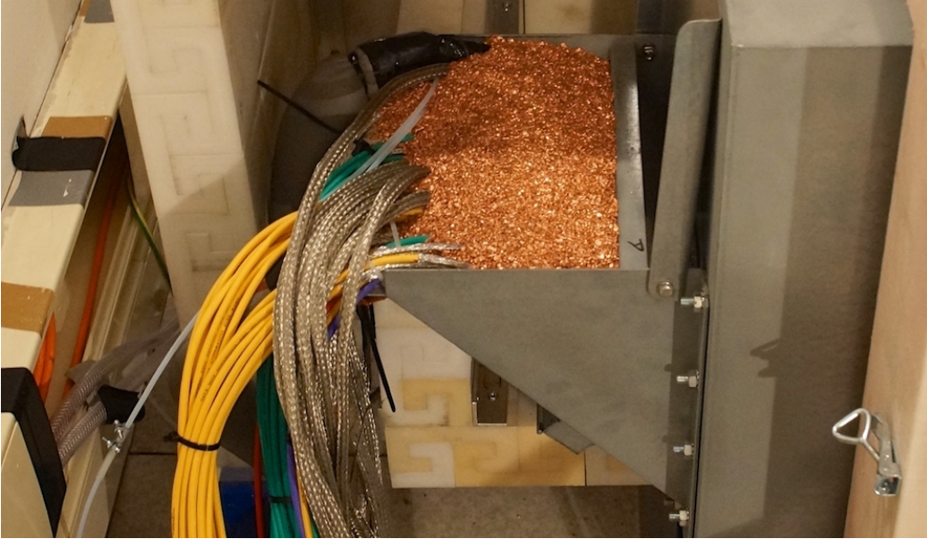
Figure A.10: The copper chute of the COBRA Demonstrator setup. The electrical isolation of the cables is removed down to the electromagnetic shielding of the cable to ensure good electric contact to the copper granulate. The green and yellow CAT6 cables are used for differential signal transmission of the detector signals, the steel meshed cables carrying the 64 high voltages and grid bias cables for the detector supply. Furthermore, supply cables for the preamplifier boxes, the cable for the pulser signals, for environmental monitoring and the cooling pipes are fed through the chute, too. The neutron shield is removed for this picture.
