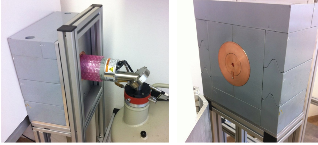
Figure 3.34: Lead collimator setup for HPGe detector of Compton scatter experiments. Beside the 5 cm lead shielding, the detector is screened by a 1 cm thick copper shroud. The frontside of the shroud can be narrowed by 2 cm thick copper plugs. Here, the copper plug with the 1 cm drill hole is installed.
