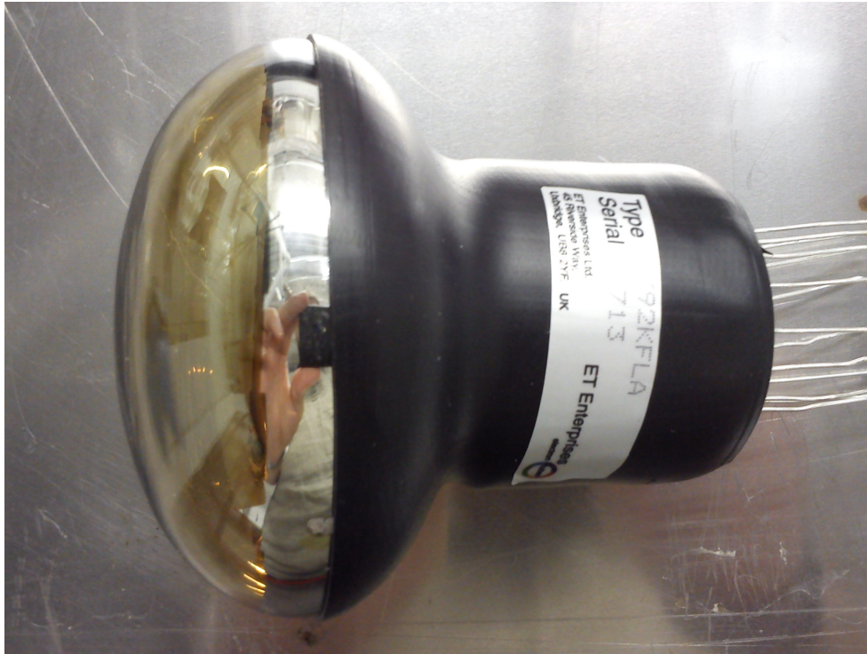
Figure 4.1: Picture of an 80 mm photomultiplier tube tested at ECAP. Taken by the author on 22 July 2013 during the assembly of the lower half of a DOM.
