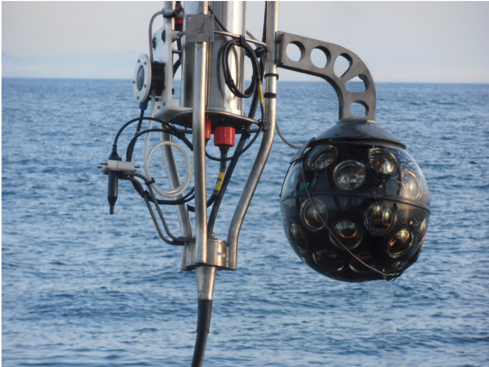
Figure 4.3: Picture of the PPMDOM, taken during deployment at the ANTARES site. Note the customised holding structure and the proximity of the local control module. The shadow cast onto the PMTs by these obstacles will be visible in the data.
