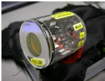
Figure 5. Picture of gaseous PMT and schematic principle of operation, which is developed in Yamagata Univ., TMU and HAMAMATSU. Photo electrons in gas are multiplied by glass capillary and metal mesh.
