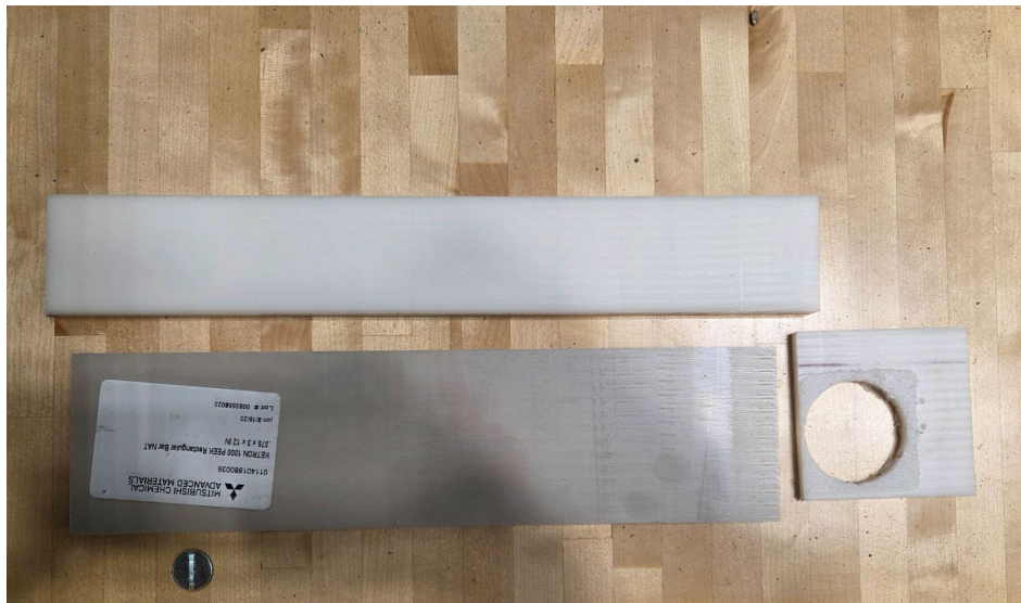
Figure 5.4: Raw material stock used for gear manufacturing showing PEEK rod (gray) and Delrin rod (white) along with a machined test piece for the end plates.
