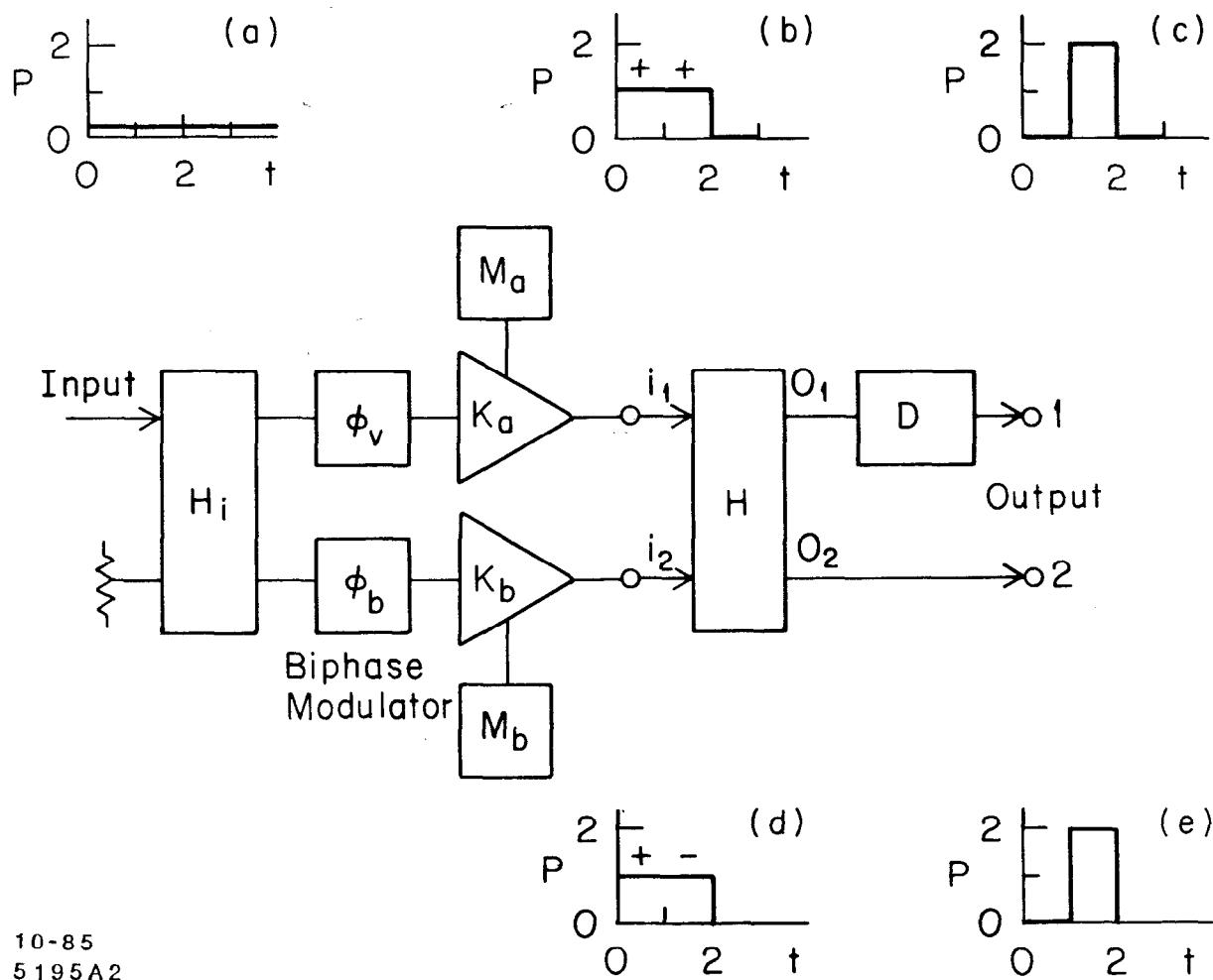
Figure 1. Diagram of a single stage BPM.
