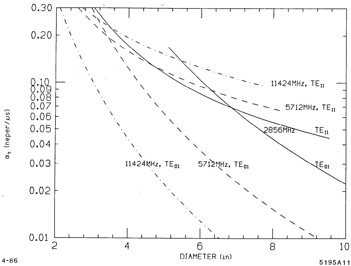
Figure 4.  $TE_{11}$  and  $TE_{01}$  attenuation as a function of diameter.
