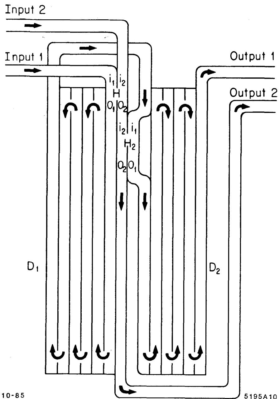
Figure 5. Two BPM stages using folded delay lines.
