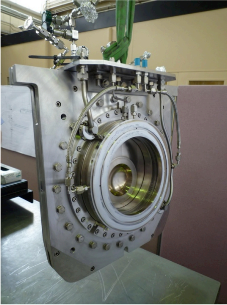
T2K window Ti-6Al-4V
