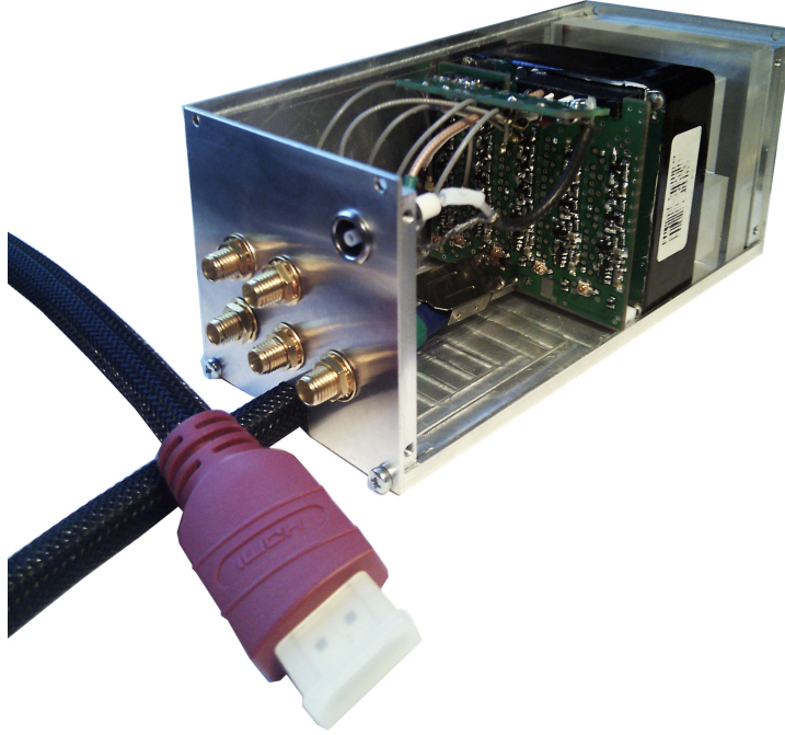
Figure 10.11: Prototype of a detector module based on XP85012. Part of the outside cover is removed to show the rear side of the sensor with front-end electronics attached. This prototype has the quartz radiator and the anode divided into 4 equal sectors.
