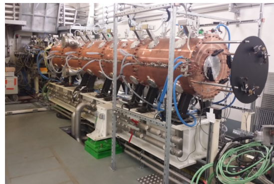
Figure 8: RFQ during the bead pull measurements.
