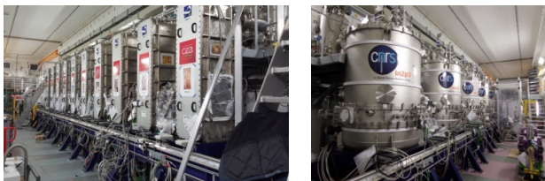
Figure 10: Cryomodules in the LINAC tunnel.
