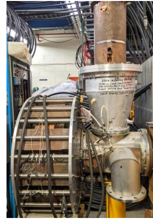
Figure 6: 50 MHz accelerating cavity with on-axis tuner.
