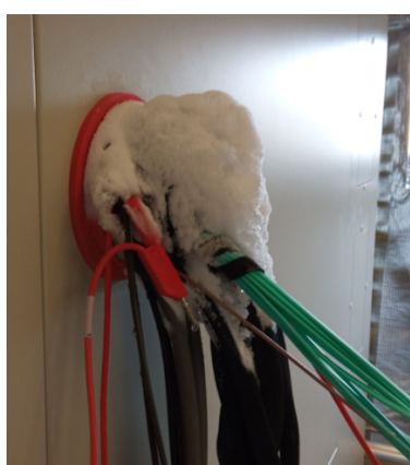
(b) Ice from air leakage
