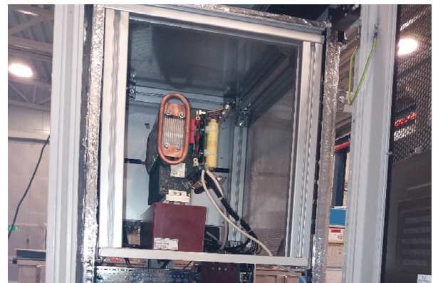
Figure 3: HV Switch in the ESS modulator prototype.
