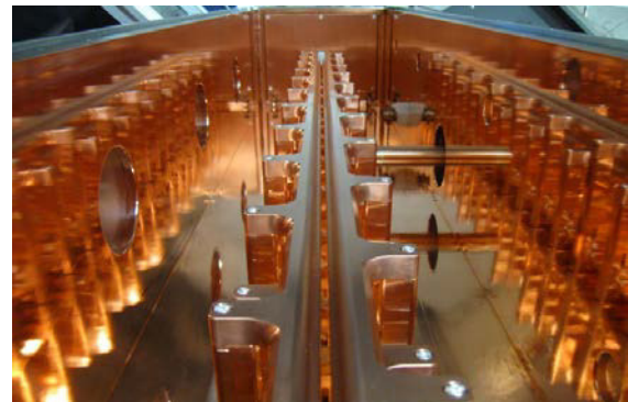
Figure 4: Interior view of the RFQ. The tuning plunger can be seen in the upper-right quadrant of the picture.
