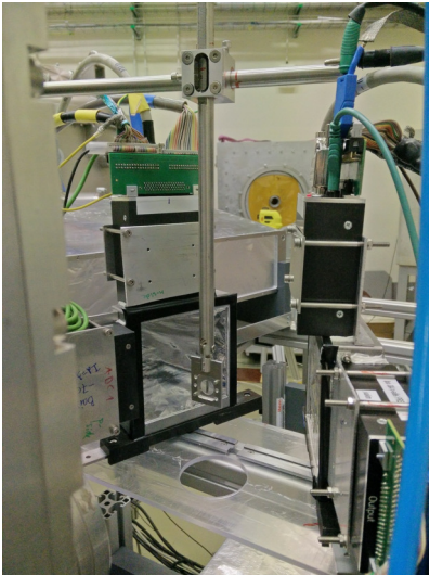
Figure 4.7.: The LYCCA DSSSDs with their two preamplifiers respectively as installed during experiment (a) and a more detailed view on the silicon waver (b).
