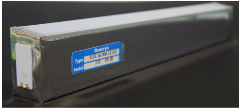
Figure 3.8.: Assembled detector unit with light tight silver taping along the gaps. The blue tag provides information on the crystal's shape and its identification number and together with the serial number of the LAAPD ensures the unique identification of the detector.
