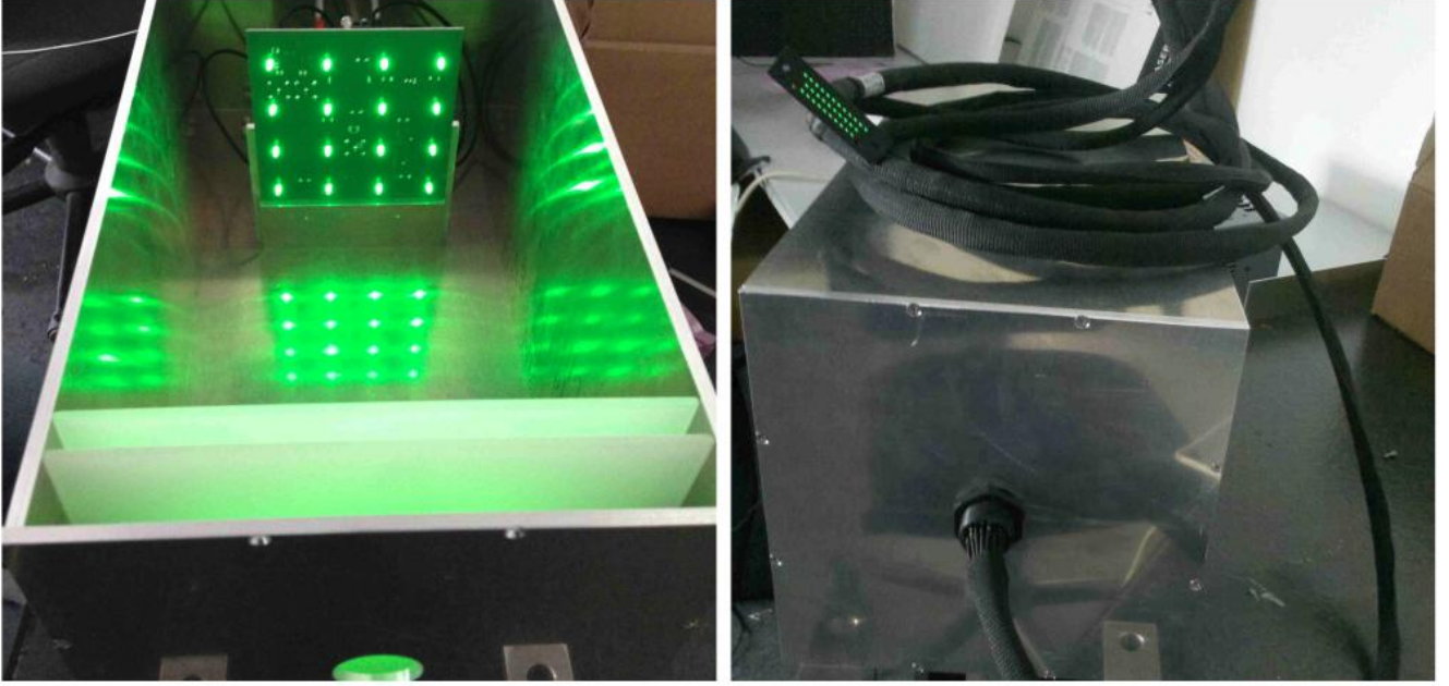
Figure 2.7.: LED source of the gain-monitoring system and the prototype of the optical-fiber transport-system ©A.Ignatov, FAIR/NUSTAR-Collaboration [24].
