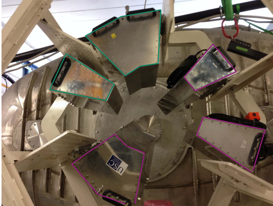
Figure 2.4.: Upstream view on the CALIFA demonstrator equipped with 7 Barrel petals, three (green) operated in high-gain mode and five (magenta) operated in low-gain mode .
