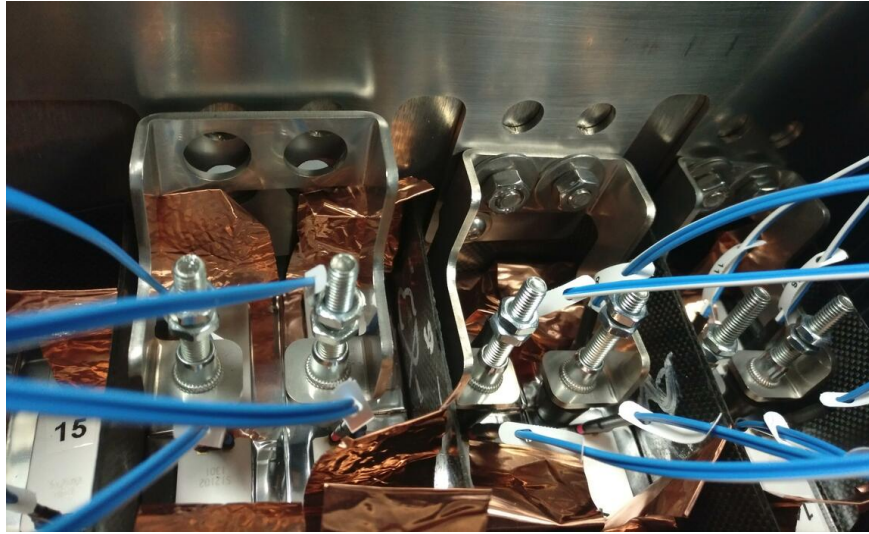
Figure 3.19.: The inner cabling of the test Iphos segment is accomplished by unshielded cabling directly plugged to the LAAPD. Adhesive copper tape is used as flaps to ensure the removability of the crystals.
