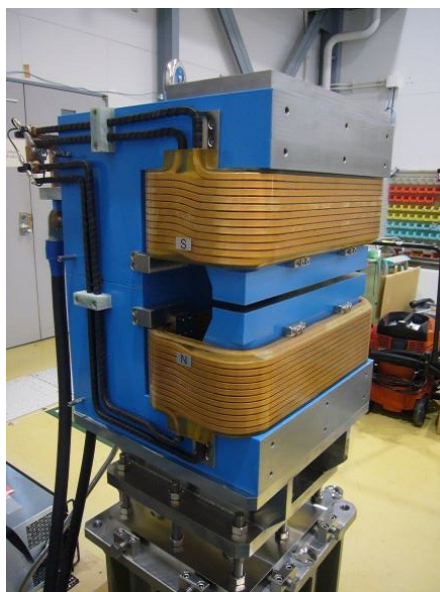
Figure 3: Picture of the DC septum magnet without the magnetic shields.
