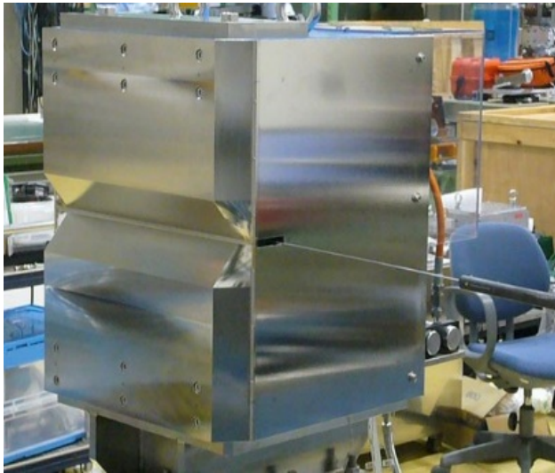
Figure 2: Picture of the DC septum magnet with the magnetic shield.
