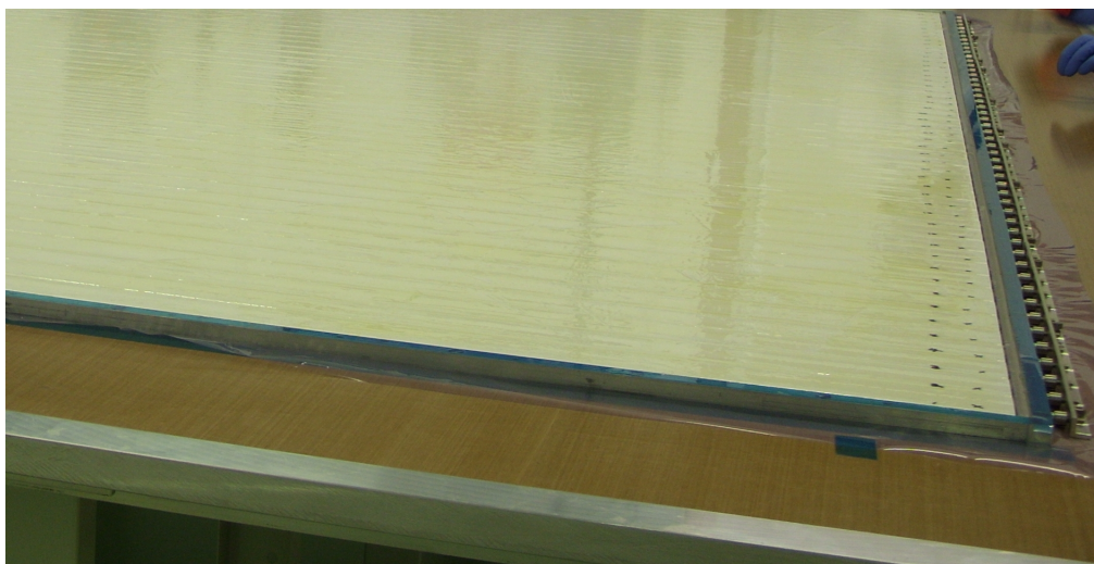
Fig. 3.13. Photograph showing a downstream ECal layer in mid-production. The figure is included in order to highlight the push-bar system, seen here on the far right. Pressure is applied to each locator pin which holds a bar in line with the frame hole and prevents glue from entering the hole during layer production.
