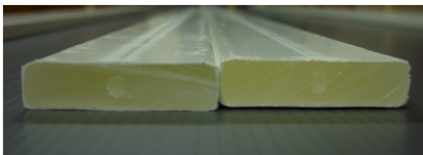
Fig. 3.11. The figure shows the oval rather than circular fibre hole that was produced in the ECal 4 cm x 1 cm cross-section bars. Image taken at Lancaster University by a member of the construction team.
