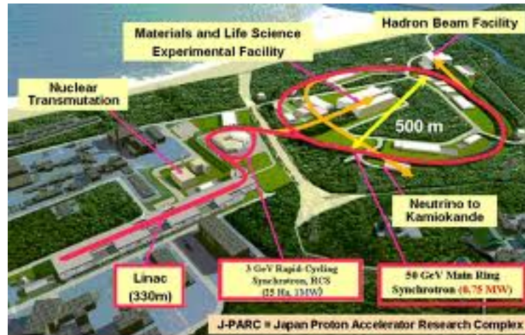
Fig. 3.2. The figure shows the layout of the JPARC Research Complex. Labelled on this figure is the design energy of JPARC's 50GeV high intensity proton beam, however during the start of the experiment and during the author's involvement with the project the beam was operating at the commissioning energy of 30GeV. Image taken from IRFU (2013).
