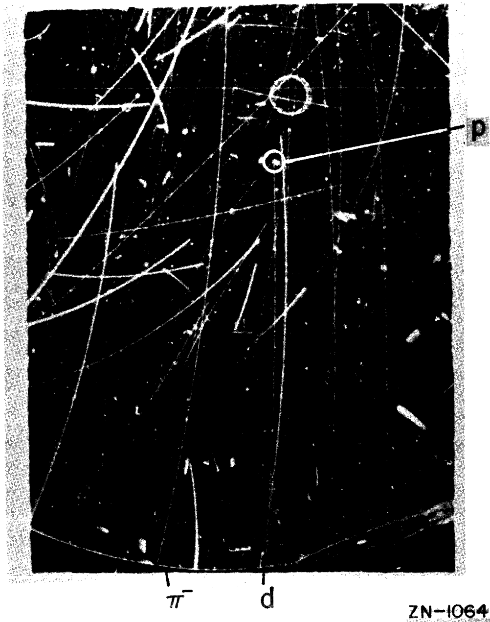
Fig. 2 Cloud chamber picture. An example of the reaction n + d \rightarrow \pi^- + p + d . The origin of the event is encircled.
