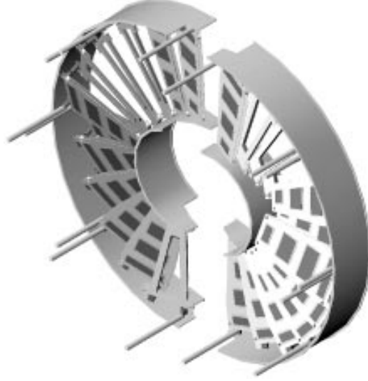
Fig. 2.51: The end-cap pixel disk structure, including service connections.
