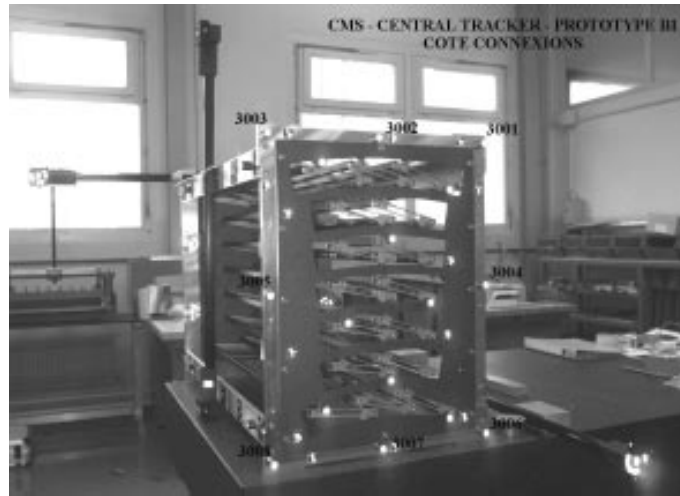
Fig. 6.28: First test setup used for evaluation of the digital photogrammetry techniques applied to the Tracker.
