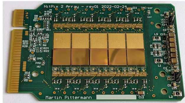
Figure 16. Picture of the 2 \times 5 matrix PCB with five mounted detectors.
