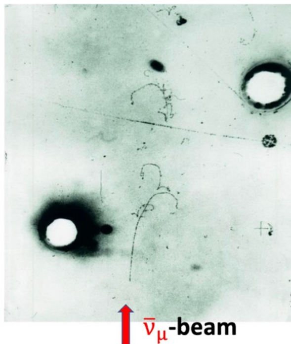
Figure 2. A single-electron event observed in Gargamelle during a \bar{\nu}_\mu run in 1971.
