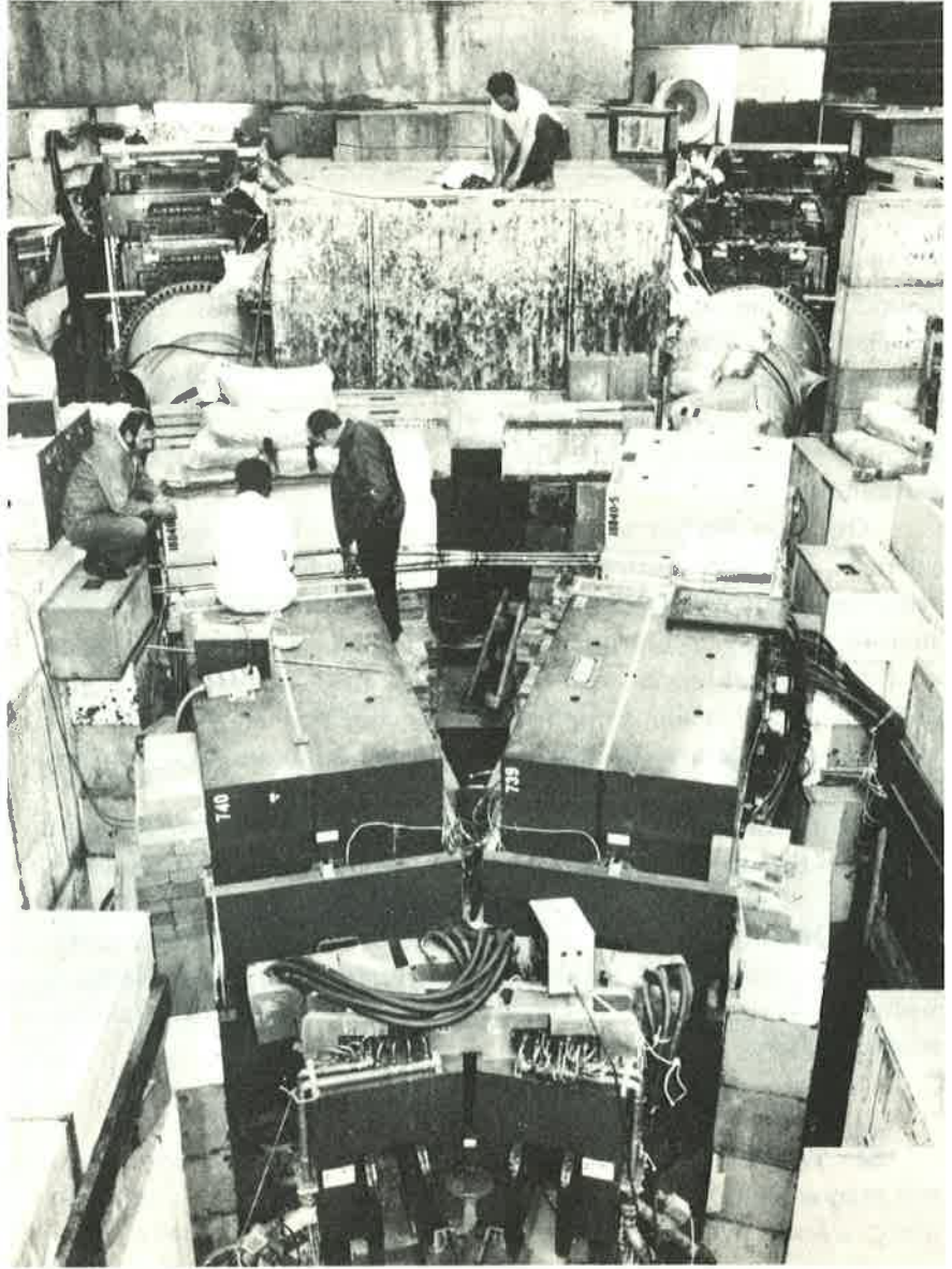
A view of the double-arm spectrometer which was used in the detection of the J particle, Brookhaven Alternating Gradient Synchrotron, 1974.
