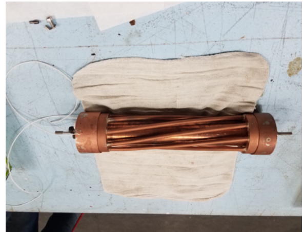
Figure 2: Ion extraction grid assembly, installed on magnetron cathode.
