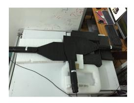
FIG. 1: Set-up with three plastic scintillator paddles for cosmic ray flux measurement.
