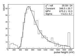
FIG. 4: Pulse height spectrum from a plastic scintillator.
