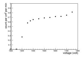
FIG. 2: 3 fold coincidence count per minute per cm<sup>2</sup> as a function of voltage.
