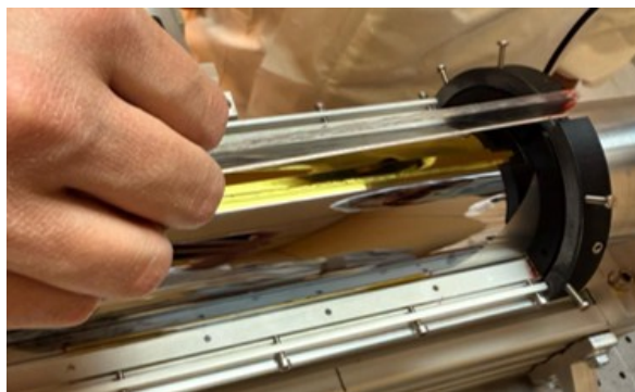
Figure 7. Central longeron placement during the local structure gluing, with the current version of the skeleton structures for holding the longerons and half rings.
