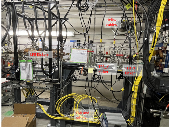
Figure 4: TFB kickers as installed in the APSU tunnel.
