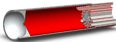
Figure 6: DECRIS-PM vacuum chamber, a hot tantalum screen is red.
