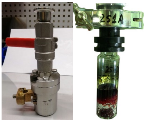
Figure 9: Containers with: left - (\text{CH}_3)_5\text{C}_5\text{Ti}(\text{CH}_3)_3 and right - \text{C}_{10}\text{H}_{10}\text{Cr} .
