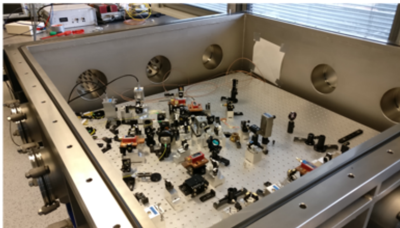
Figure 5: The optical part of the LOT in its vacuum chamber
