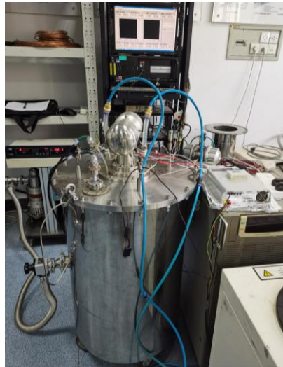
Figure 3. Photograph of the low-temperature emissivity measurement device for insulating materials developed based on a high-frequency pulse tube cryocooler.
