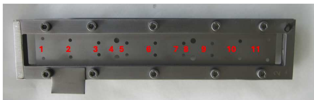
Figure 2. Top view of the coated slab surrounded by the aluminum frame used during the deposition. The holes are for the correct alignment of the slab in the waveguide during THz measurements. The red numbers are the position where the XRF thickness measurements are taken.
