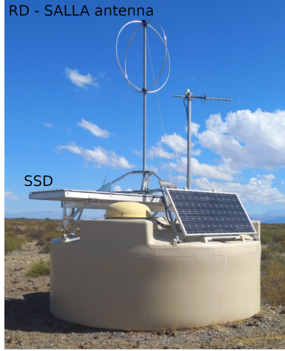
Figure 1: Photo of an AugerPrime SD station operating in the field. The visible AugerPrime enhancements are the RD - SALLA antenna and the aluminum case containing the SSD mounted on the station. Inside the station, an additional small PMT and the upgraded electronics board (UUB) are installed.
