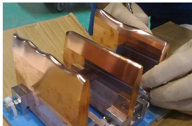
Figure 2: Test piece of the vane tip for checking the surface roughness with the machining conditions.
