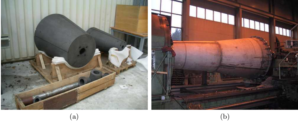
Figure 2.18: (a) Graphite and (b) steel envelope for the front absorber
