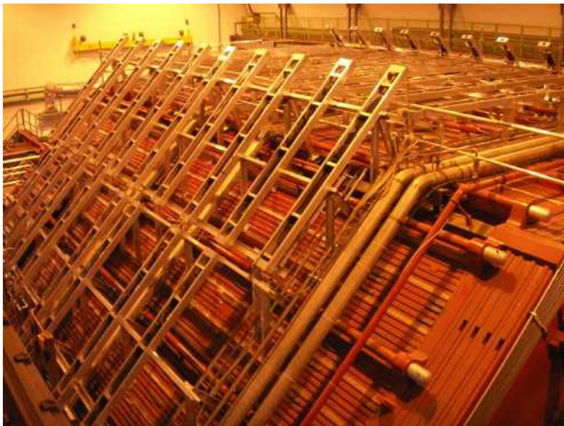
Figure 2.11: Photograph of ACORDE scintillator modules on the upper faces of the magnet yoke of ALICE.
