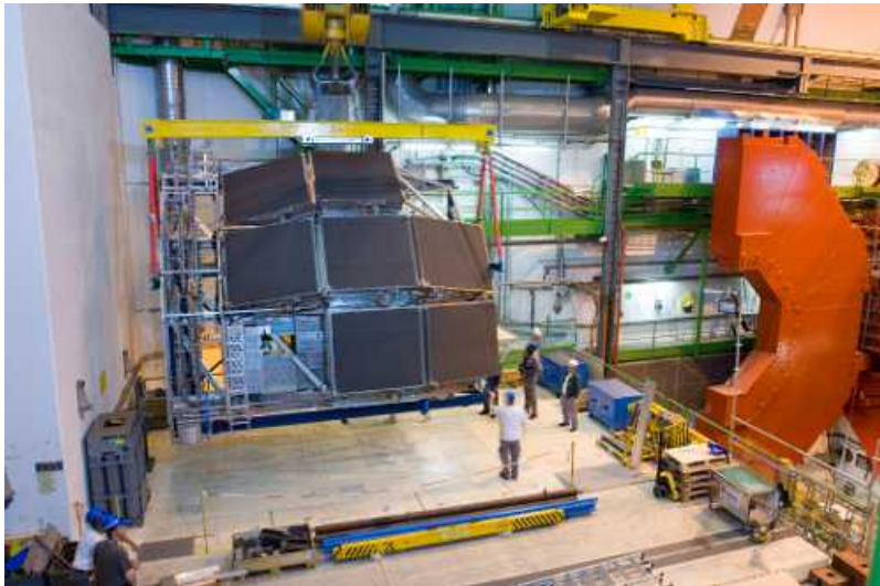
Figure 2.8: View of modules of HMPID mounted on the cradle.
