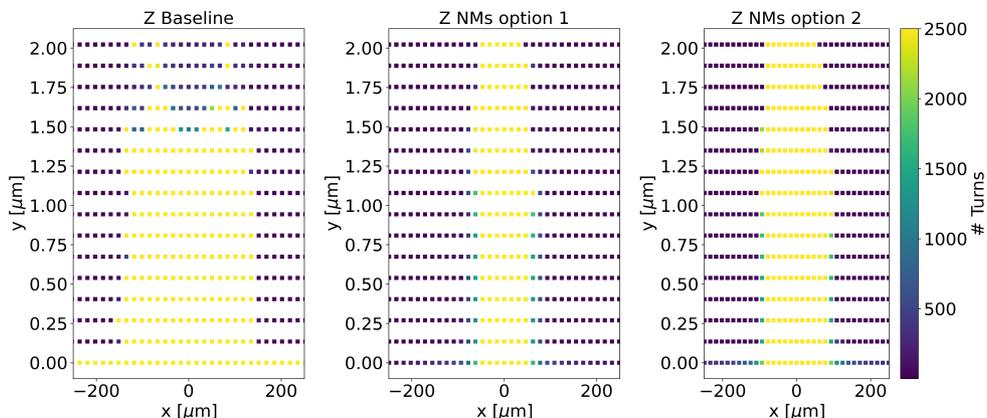
Figure 2: DA for the different lattice options at the Z energy: the baseline and the NMs lattices Options 1 and 2. The plots were obtained with the same number of turns and distribution in the X-Y space for tracking.
