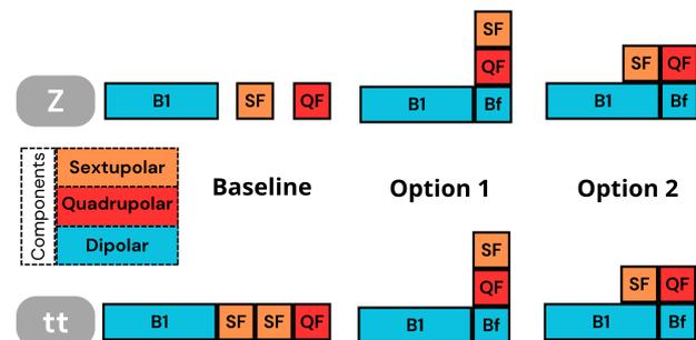
Figure 1: The two options used for studying the dynamic aperture with the implementation of NMs in the FCC-ee. Option 2 is the closest to the baseline (shown on the right of the figure) in terms of optics design. Both options 1 and 2 are feasible according to the magnet design experts.
