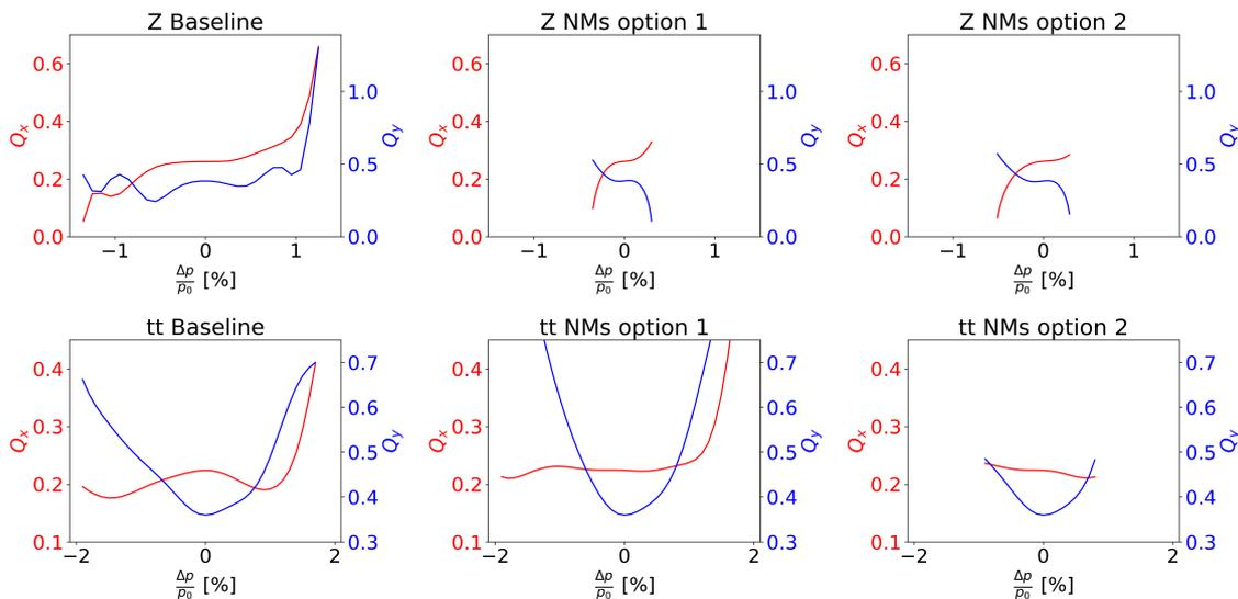
Figure 4: Horizontal and vertical fractional part of tunes versus relative momentum deviation for all the lattices.
