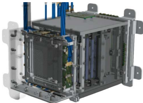
Figure 3. A CAD image of the Zirettino, displaying the four PCBs of the FTK, equipped with SiPM arrays, and the SAMTEC cables.
