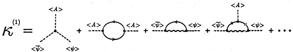
Fig.1 Some of the diagrams included in  $\kappa^{(1)}$ , which contribute to the modified Dirac equation (13). The wavy line is the photon propagator. The solid line with an arrow denotes the electron one.
