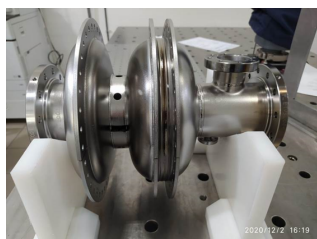
Figure 2: 1.5 cell Nb SRF gun with cooling rings welded.
