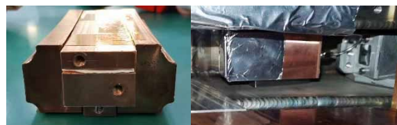
Figure 13: Probe with radial fingers used for the commissioning of ESDs (left) and self-shielded probe for the commissioning of MCs(right).
