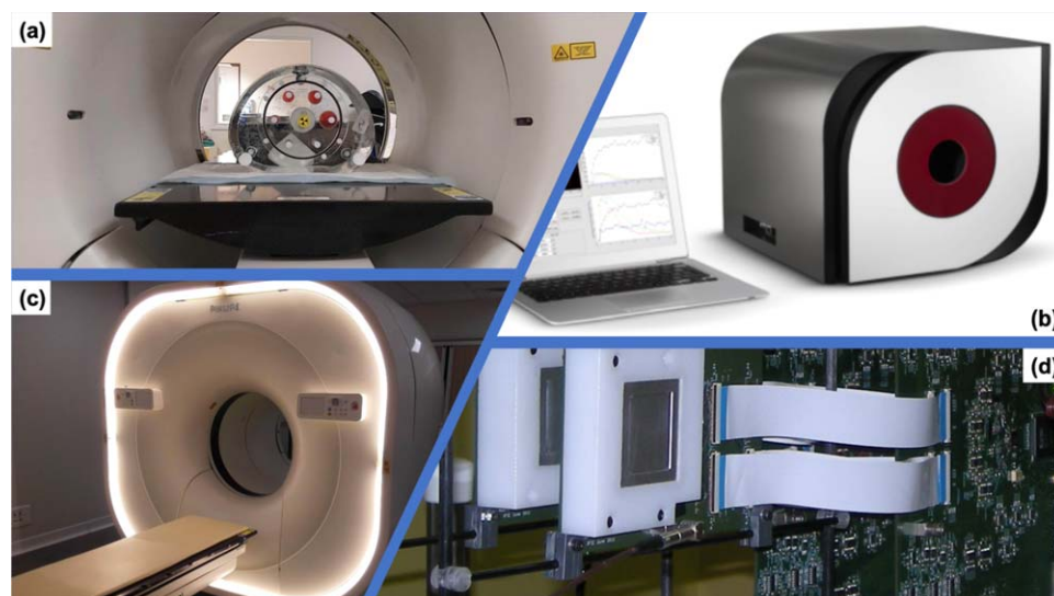
Figure 2. Examples of some simulated imaging systems (clinical, pre-clinical, prototype). (a) NEMA IEC Body Phantom Set ready to be imaged on a PET/CT. (b) The Bioemtech \gamma -eye preclinical device. (c) Philips Vereos Digital PET/CT; (d) MACACO Compton Camera prototype with 2 layers of \text{LaBr}_3 monolithic crystals coupled to SiPMs, developed by IFIC-Valencia. Reproduced with permission from Philips France Commercial.
