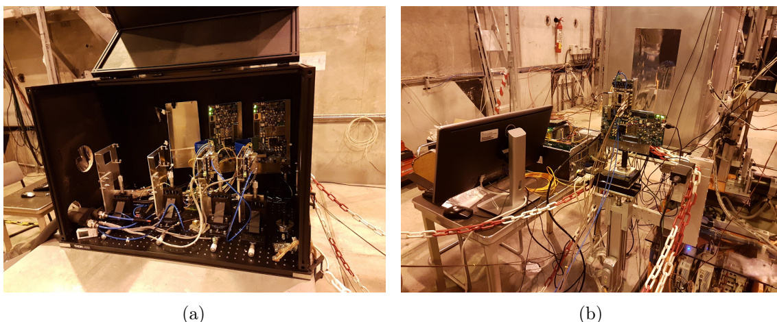
Figure 5.10.: 5.10a : The box with planes 1 and 2 of TDCPix, close together. Picture taken during the test beam in 2017. 5.10b : The TimePix3 telescope (gray box) and plane 3 of TDCPix ("L" structure in front of it). Picture taken during the test beam in 2017.
