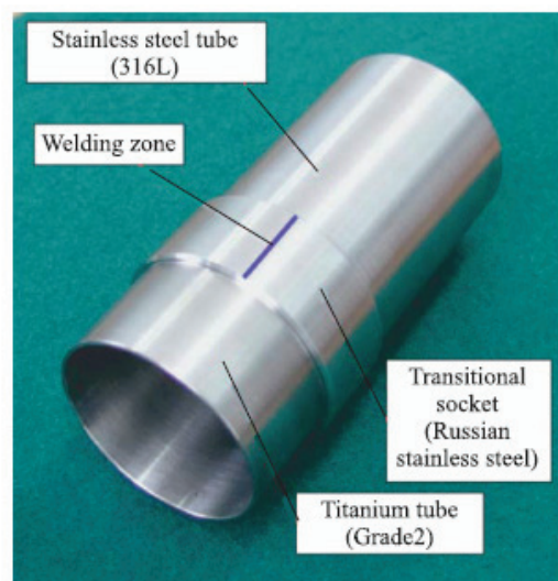
Figure 2: Ti+SS transition element.
