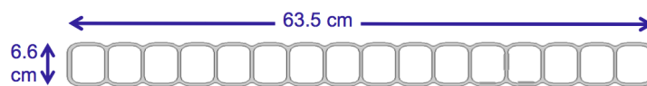
Figure 3.9: An end on view of an extrusion consisting of 16 NOvA cells. Taken from [43].
