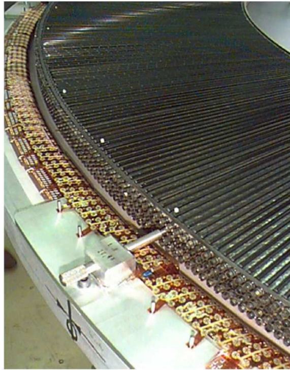
Fig. 2.14: Photograph of TRT endcap wheel during assembly. The inner and outer C-fiber rings can be seen, as well as the first layer of straws and the first stack of polypropylene radiator foils beneath it [3].
