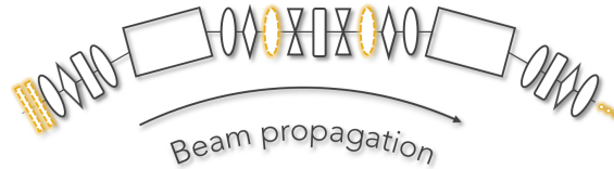
Figure 2. Scheme of a right turning DBA. Black parts are present in all the DBAs, the golden parts are the elements present only in the 14 th DBA that controls the dispersion leak, the final three dots represent the remaining 7 quadrupoles of the the matching line.
