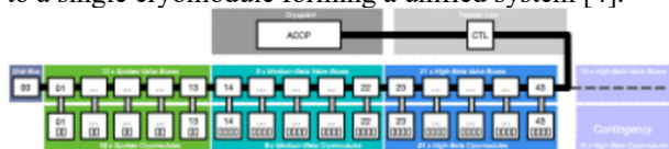
Figure 1: Layout of the accelerator cryogenic system.
